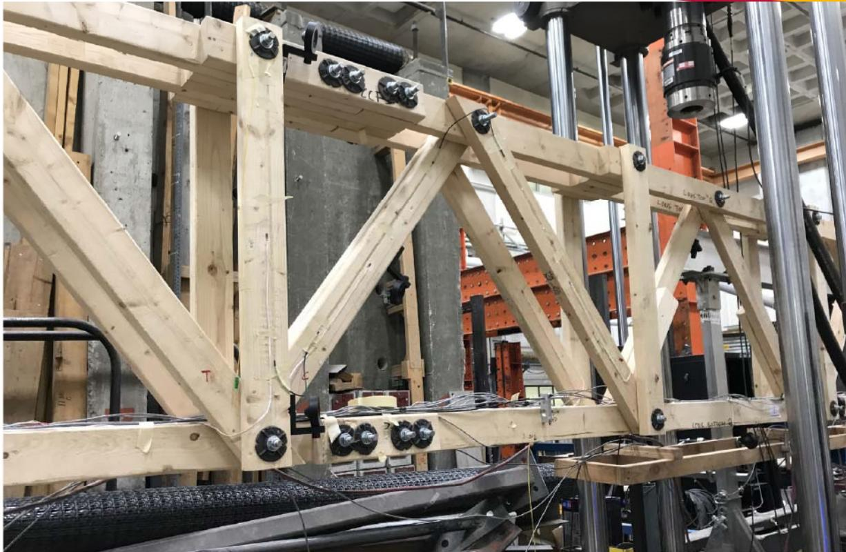
DOS instrumented warren truss (RMC structures lab)
